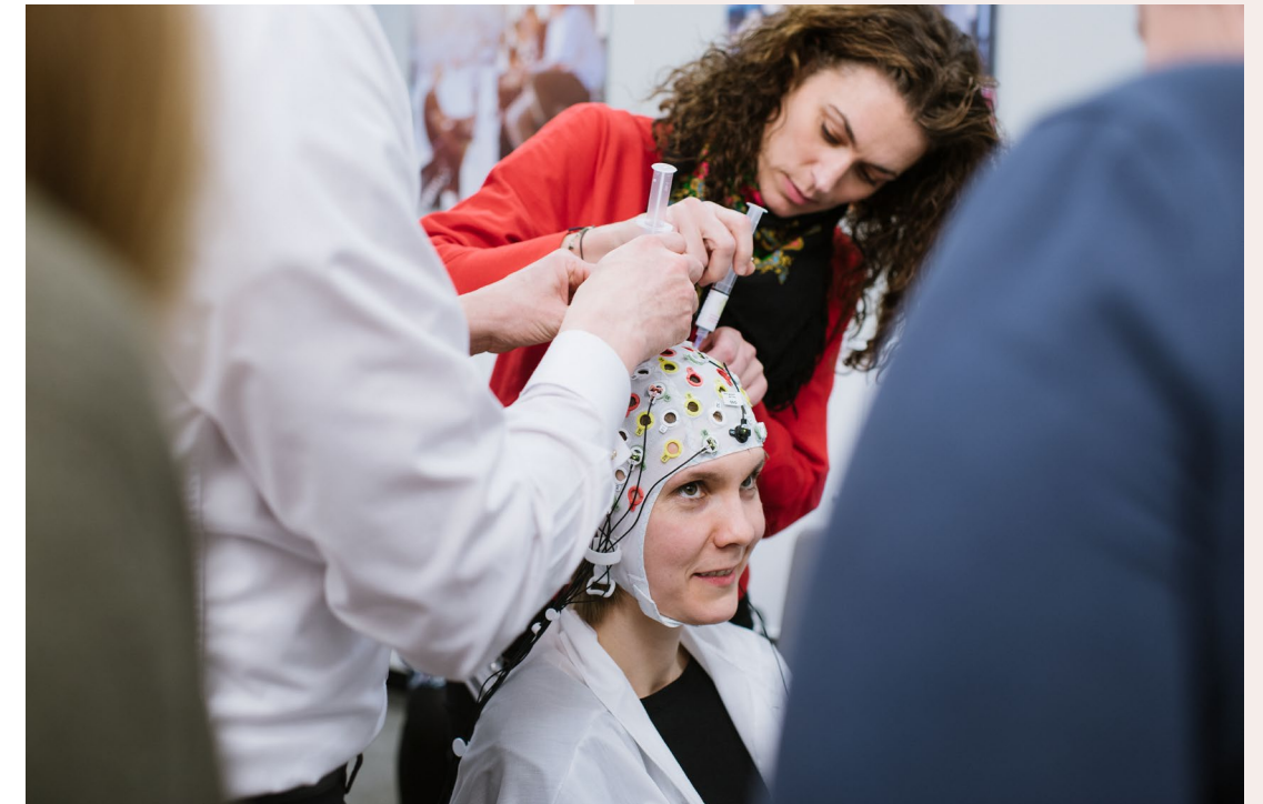
Testing of the new EEG equipment, which records electrical activity in the brain. The syringes may look dramatic, but are only used to apply conductive gel, ensuring good signal quality.
